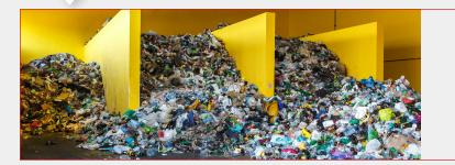
After being deposited correctly, the waste is collected, sorted and pre-treated to remove impurities, and then processed for efficient use in cement-making.
